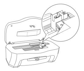
3. Open the document cover and slide the carriage lock lever, as shown in the illustration below, to lock the scanner carriage.
